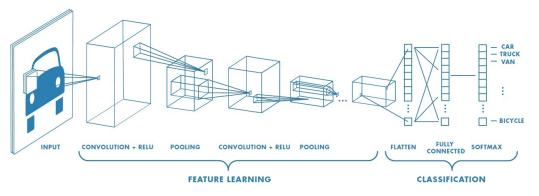
The "depth" dimension in the layers shown as cuboids corresponds to the number of channels in the output tensor. (Figure source: https://www.mathworks.com/solutions/deeplearning/convolutional-neural-network.html)
