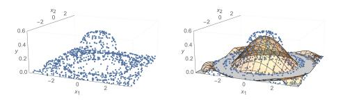
The raw data (with n = 1000 random samples) is plotted on the left, and the regression result (curved surface) is on the right.
