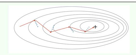
The red arrows show the update after each successive step of mini-batch gradient descent with momentum. The blue points show the direction of the gradient with respect to the mini-batch at each step. Momentum smooths the path taken towards the local minimum and leads to faster convergence.
