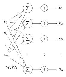
Since each unit has a vector of weights and a single offset, we can think of the weights of the whole layer as a matrix, W, and the collection of all the offsets as a vector  $W_0$ . If we have m inputs, n units, and n outputs, then
