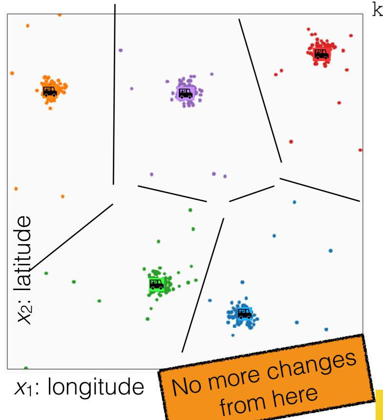
k-means  $(k, \tau)$ Init  $\{\mu^{(j)}\}_{i=1}^k, \{y^{(i)}\}_{i=1}^n$ for t = 1 to  $\tau$  $y_{\text{old}} = y$ for i = 1 to n  $\arg\min_{i} \|x^{(i)} - \mu^{(j)}\|_{2}^{2}$ for j = 1 to k  $\frac{\sum_{i=1}^{n} \mathbf{1} \{ y^{(i)} = j \} x^{(i)}}{\sum_{i=1}^{n} \mathbf{1} \{ y^{(i)} = j \}}$ if  $y = y_{\text{old}}$ break return  $\{\mu^{(j)}\}_{i=1}^k, \{y^{(i)}\}_{i=1}^n$
