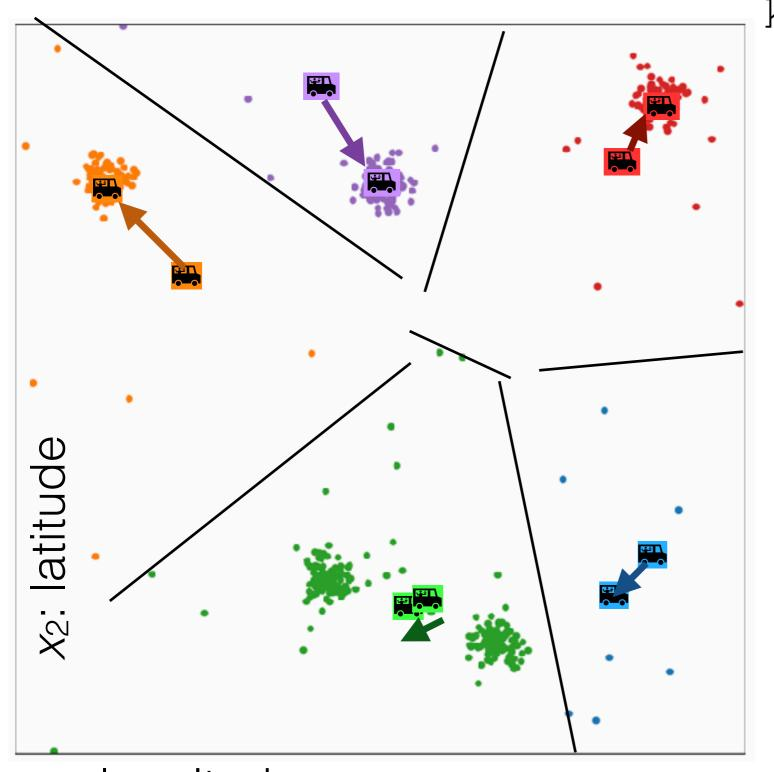
k-means  $(k, \tau)$ Init  $\{\mu^{(j)}\}_{j=1}^k$ for  $t = 1 to \tau$ for i = 1 to n  $\arg \min_{j} \|x^{(i)} - \mu^{(j)}\|_{2}^{2}$ for j = 1 to k  $\frac{\sum_{i=1}^{n} \mathbf{1} \{ y^{(i)} = j \} x^{(i)}}{\sum_{i=1}^{n} \mathbf{1} \{ y^{(i)} = j \}}$
