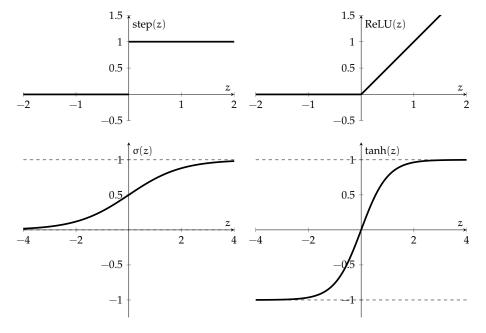
The original idea for neural networks involved using the **step** function as an activation, but because the derivative of the step function is zero everywhere except at the discontinuity (and there it is undefined), gradient-descent methods won't be useful in finding a good setting of the weights, and so we won't consider them further. They have been replaced, in a sense, by the sigmoid, ReLU, and tanh activation functions.
